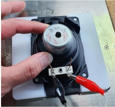
Insert Unit to JIG & connect cable
